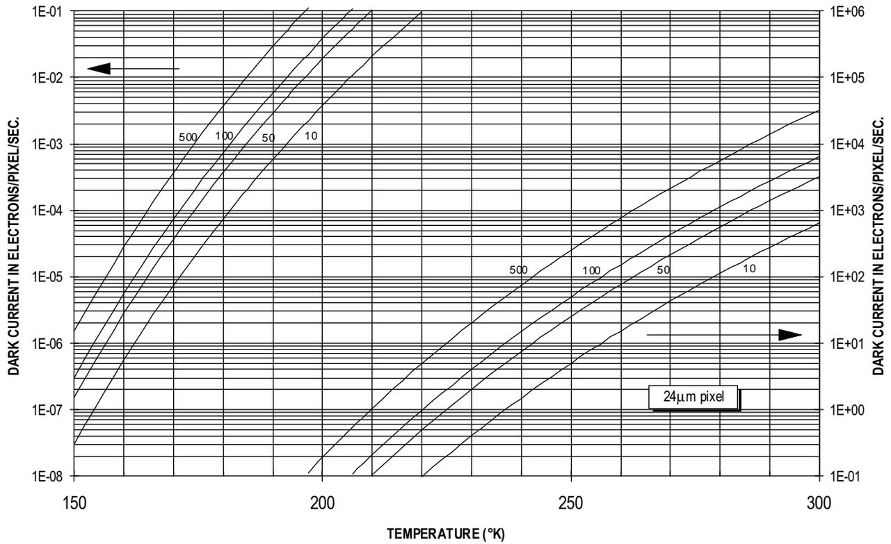
FIGURE 8 Effect of temperature on dark current. Parameter is pAmp/cm<sup>2</sup> at 293K
