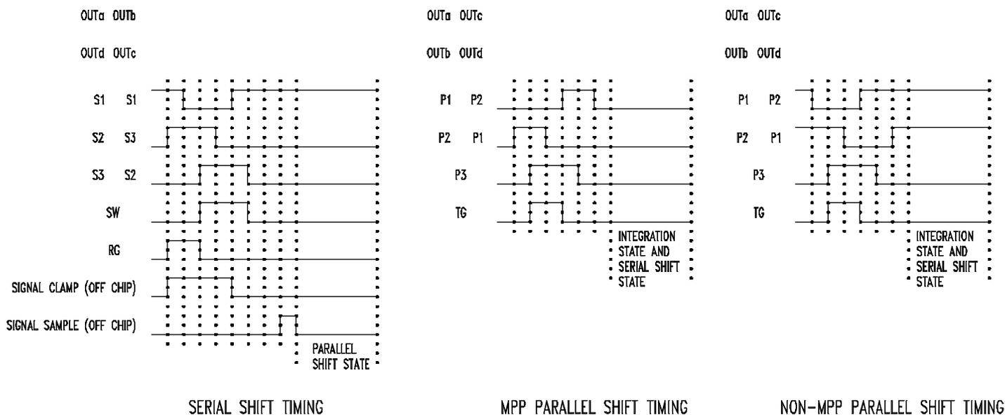
FIGURE 3 Serial and Parallel timing for all outputs
