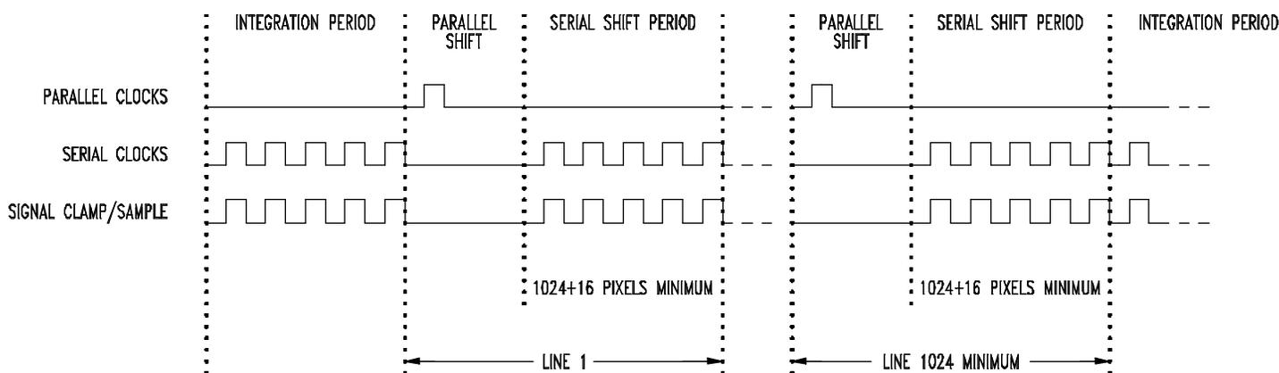
FIGURE 4 Typical full-frame readout
